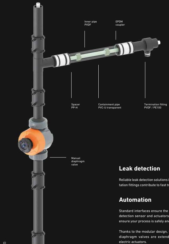
Reliable leak detection solutions in combination with segmentation fittings contribute to fast troubleshooting.
